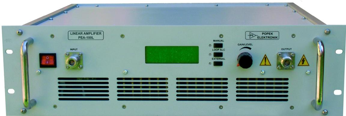
PEA-100L is a linear, broadband telecommunication and, broadband high power amplifier (100 W) making use of automatic measurement systems, broadband telecommunication and laboratories. The broadband and high gain enable the amplifier to gain signals from typical signal generators. After calibration the amplifier with antenna systems are used for generation of electromagnetic measurement fields. The device enable signal transmission with the following modulations: AM, FM, SSB and pulse.
